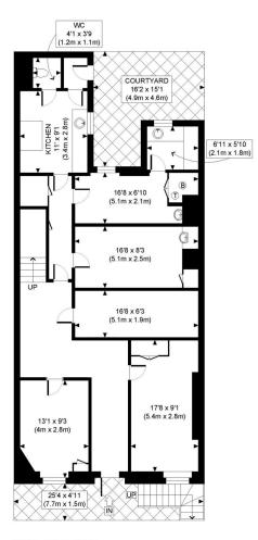
LOWER GROUND FLOOR GROSS INTERNAL NET FLOOR AREA 798 SQ FT GROSS FLOOR AREA 1169 SQ FT
